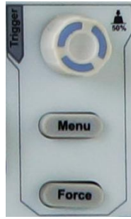
Figure 3-13 Trigger Control Zone
