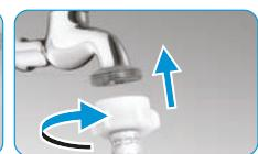
1. Check the availability of the rubber gaskets on both sides of the flexible tube. If necessary, insert the rubber gaskets into the threaded fittings of each hose end for sealing the connections.
