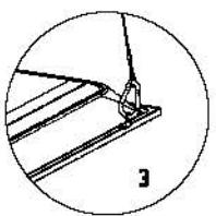
The product should be installed with safety cable.
