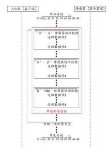
The host computer (client) sends a "start data frame" to the sensor (server), and the sensor returns measurement data of 20°-340° in several frames.
