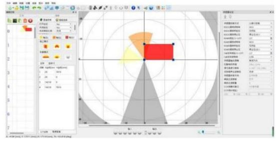
Part 4: Channel detection graphics output 1, output 2, output 3 editing mode. Independent mode: under independent mode, irregular shapes, sectors and rectangles can be set separately. The irregular shapes are composed of up to 100 points of connected lines.
