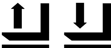
The lifting button and the lowering button are located on both side surface of the middle control handle. Press the lifting button, and the forks move up; press the lowering button, the forks go down.
