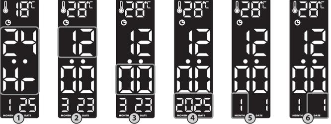
**1** Press the **"MODE"** button to select the time display mode. You can choose a 12-hour format or a 24-hour format. Control the options using the **"▲"** and **"▼"** buttons.
