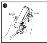
Rotate the flush valve body to separate the body from base as shown in the Fig.
