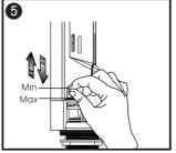
When moving the red adjusting piece from bottom to top, the full flush volume decreases gradually, The adjustable distance is 20mm(13-16").
