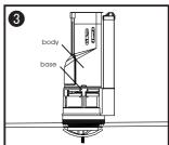
Install the flush valve body on the base again, rotate it to a proper position and lock.
