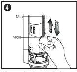
When moving the partial flush float from bottom to top, the partial flush volume decreases gradually, The adjustable distance is 60mm(2-1/4").
