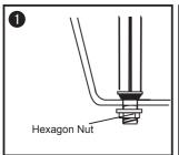
Spin the hexagon nut open and put the fill valve into the water-in tank hole, make sure the filter are at the position as shown, screw the hexagon nut tight.
