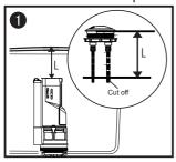
"L"must be measured just as showed in figure. To cut off the excess length of the rod.
