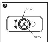
Install the flush valve base into the outlet to make the "U" clasp can clip on the tank properly. Rotate the base to choose proper angle and lock the screw.
