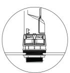
Flush valve can also be used in tow-piece tank.
