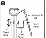
Rotate the adjustable rod 90 degree and draw out, move the fixed ring to adjust the float height and water level. Press the inner float, adjustable rod to the lowest position, put the rod back into the inner float, then rotate and fix it.
