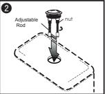
Cut the adjustable rod to a proper length, put the push button into the hole.
