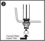
Drain out of the water supply tube clean and connect the water supply tube
