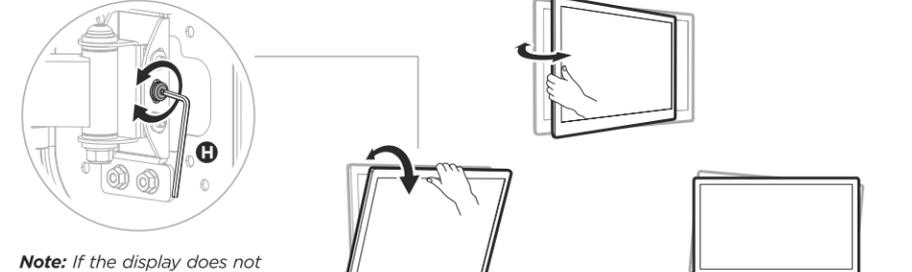
**Note: If the display does not stop at your desired position, adjust the screws as shown.**
