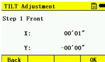
3. Press (OK), collimate the same target in the reverse position
