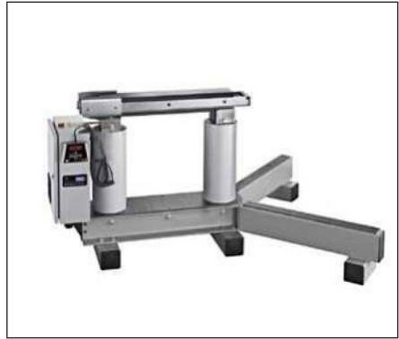
Figure 2: TIH L after bearing supports assembly
