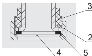
Type C — blind connection: the plug is formed from the union nut (2) and the washer (4) and screwed onto the ring (3) with the O-ring (5).
