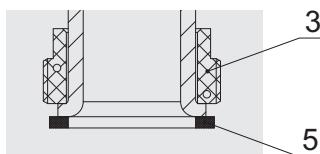
Type B is a ring with  $1\frac{1}{2}$ " male thread (3) with a flat O-ring (5), used to connect the hydraulic separator PROFACTOR® PF PU 1054.
