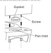
4 Connect the supply hose to the cistern inlet and feed the hose through the appropriate side hole in the pan.
