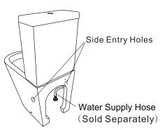
**5** Connect the supply hose to the shut-off valve to test the system for leaks. Shut off the water supply and disconnect the hose. Insert a capping plug into the unused hole.
