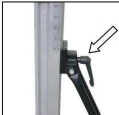
Loosen the clamp lever on the bracing.
