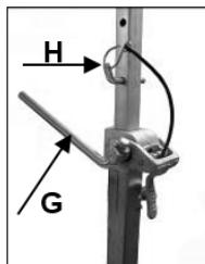
Position the drill rig. Place the quick action bracing unit as close as possible behind the column on the base of the rig. Fix the drill rig by turning the crank (G) clockwise. Secure the position by means of the appropriate bolt (H).
