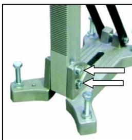
Loosen both Allen screws M10 with the enclosed wrench SW 8
