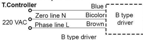
Note: the zero line of valve shall be same as temperature controller
