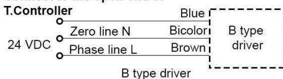
Note: the zero line of valve shall be same as temperature controller
