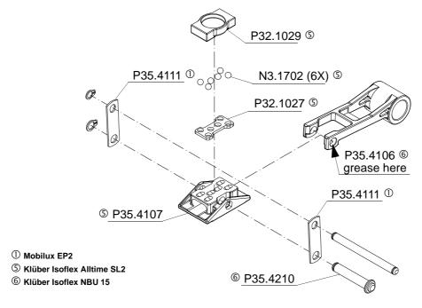
All other parts have to be lubricated according to the explosion drawing. Lubrication interval: While each maintenance or after 12 months at the latest.
