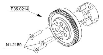
The screws N1.2189 have to be glued additionally in the wheel P35.0214 using **LOCTITE 222.**
