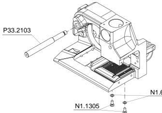
The bolt P33.2103 has to be glued into the housing P33.2102 using **Loctite 603**.
