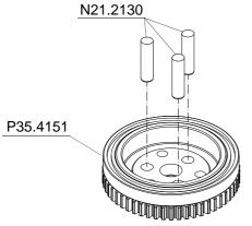
Gear wheel P35.4151 and parallel pins N21.2130 have to be glued with **LOCTITE 603**
