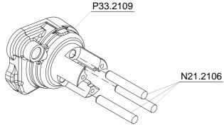
The parallel pins N21.2106 have to be glued into the gear body P33.2109 using **LOCTITE 603**.
