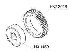
The Bearing N3.1159 has to be glued into the gear wheel P32.2016 with **LOCTITE 603**.
