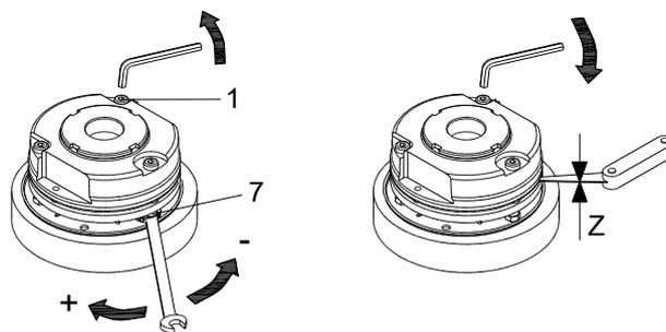
In general working condition, the first air gap adjustment should proceed after brake working for 1500~2000hours, frequency of air gap adjustment is every 6 months. In severe working condition, like frequently brake, repeatedly sudden brake, the first adjustment can be shortened and adjust the interval.
