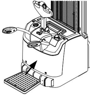
There install main parts as hydraulic unit, main drive unit and electric system etc. under the hood. When check or maintain, please open the rear hood.
