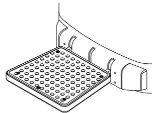
This pedal can be folded so that you can put down the pedal and stand on it when operating the truck for a long distance. When transporting at a narrow space, folding the pedal, stand on ground to operate the truck.
