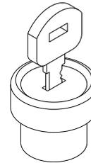
Turn on the key switch, and the power is on. Turn off the switch, and the power is off. Turn off the key switch before charging.
