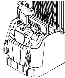
When check battery, take out the plug, charge or replace the battery, you can easily open the battery cover.
