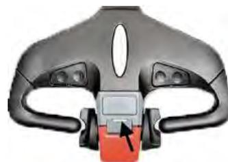
When this light is on, the truck is in low speed mode.
