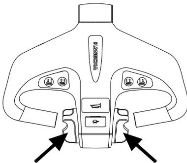
This button is at both sides of control lever head, one linkage per left and right. It is to control travelling direction and travelling speed.
