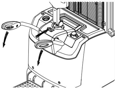
When open the arm guard, push the arm guard lock switch with one hand and the other hand lift up the arm guard until it rotates to certain angle, release arm guard lock switch and lift the arm guard to lock position.
