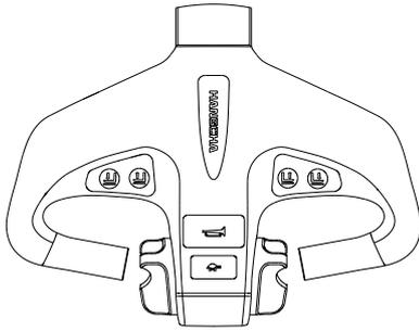
Control truck steering and braking.
