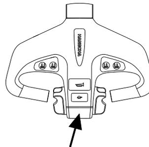
This switch is at the head of control lever, once touch this button, the truck moves forward. It is used to protect people from being clamped by the control handle.
