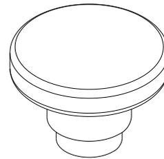
Press this switch, power is off. Press it when emergency or no use. If re-start needed, pull upward.
