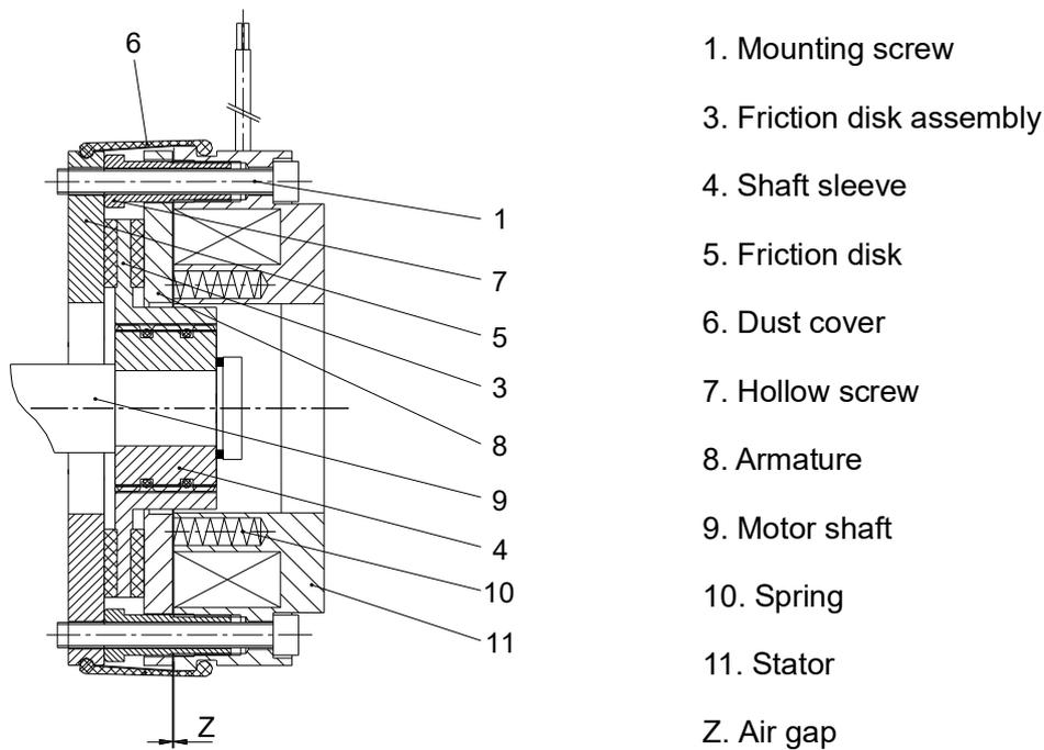
Fig.2-5 Structure chart of electromagnetic brake
