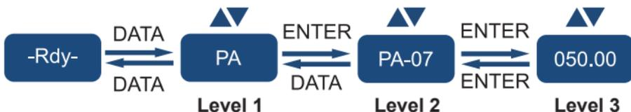
The operation panel adopts a three-level menu structure. Function parameter group (level 1 menu) → function code (level 2 menu) → function code setting value (level 3 menu).
