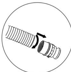
Screw the vacuum tube into the front to match the internal thread
