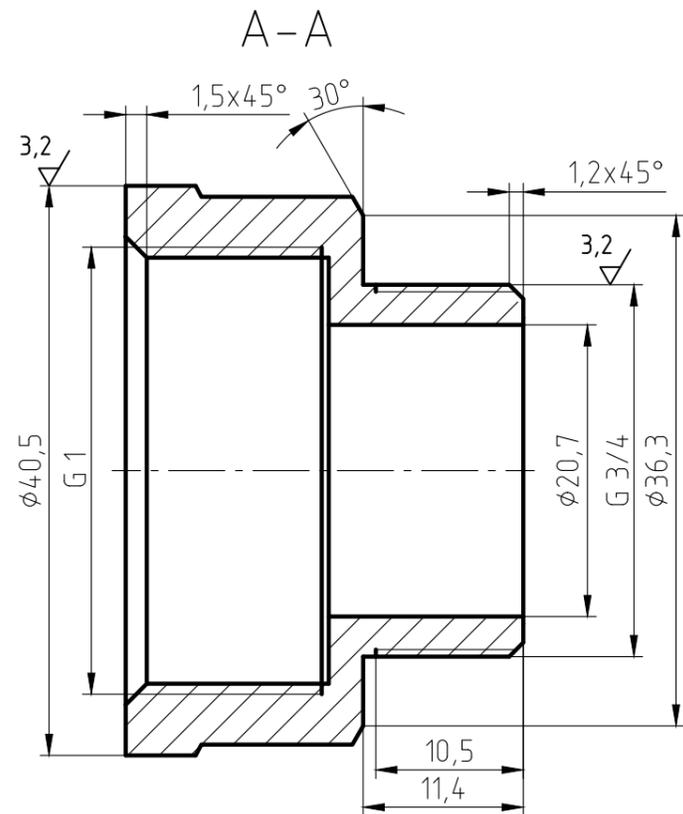
1. The parts should be 59-1 materials, no fissures surface sand-throwing treatment and nickel plating. All nickel plating.
