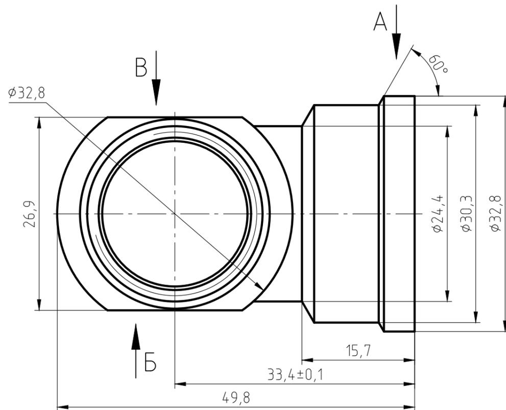
1. The parts should be 59-1 materials, no fissures surface sand-throwing treatment and nickel plating. All nickel plating.
