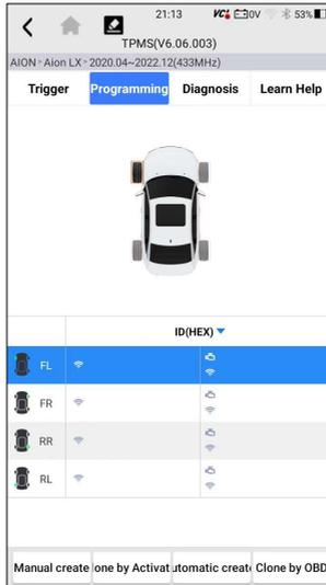
Figure 11-11 Sample Manual Create Function Screen
