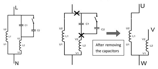
U1 and V1 are the common terminals of the windings. Connect them to the output terminal W of the solar pumping inverter. Connect U2 to the output terminal U of the inverter. Connect V2 to the output terminal V of the inverter.
