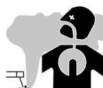
The fumes, gases and dust produced during welding are hazardous. It is mandatory to ensure adequate ventilation and/or extraction to keep fumes and gases away from the work area. An air fed helmet is recommended in cases of insufficient air supply in the workplace. Check that the air intake is in compliance with safety standards.
