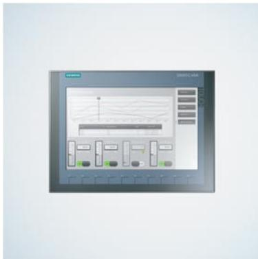
SIMATIC HMI, KTP1200 Basic DP, Basic Panel, Key/touch operation, 12" TFT display, 65536 colors, PROFIBUS interface, configurable as of WinCC Basic V13/ STEP 7 Basic V13, contains open-source software, which is provided free of charge see enclosed CD
