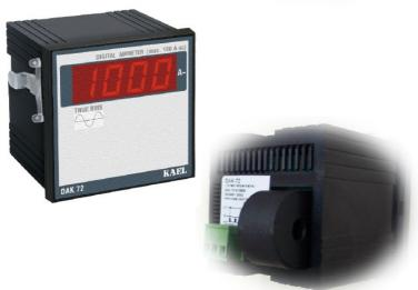
Designed for industries that do not have much spare places in there current transformers or to reduce the costs. It contains a small current transformer. It measures the current in the cable that will be passed through a hole in the current transformer.
