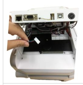
After opening, pull out the wire just put into the hole and insert it into the wafer 1x7P P1.25 connector on the main board
