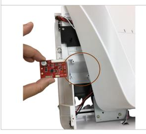
5. After opening, insert this cutter board and lock the cutter board with two screws
