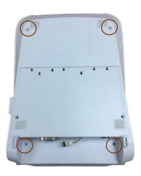
4. Turn the printer upside down, remove the four screws located on the bottom cover, and open the bottom cover
