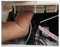
Open the small cover, insert the wafer
