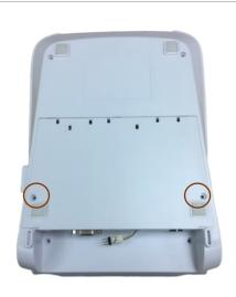
4. Turn the printer upside down, remove the two screws located on the bottom cover, and open the bottom cover
