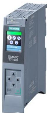
SIMATIC S7-1500, CPU 1513-1 PN, central processing unit with working memory 300 KB for program and 1.5 MB for data, 1. interface: PROFINET IRT with 2 port switch, 40 NS bit-performance, SIMATIC memory card necessary
