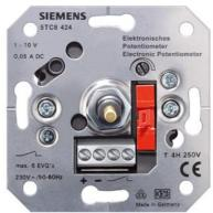
electronic potentiometer with pushbutton off switch 6 A FM, 1-10 V control input 0.04 A Screw terminals for claw and Screw mounting
