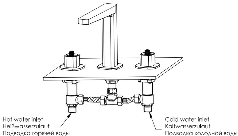
Connect the hot and cold water inlet. Make sure there is no leaking in the connection.
