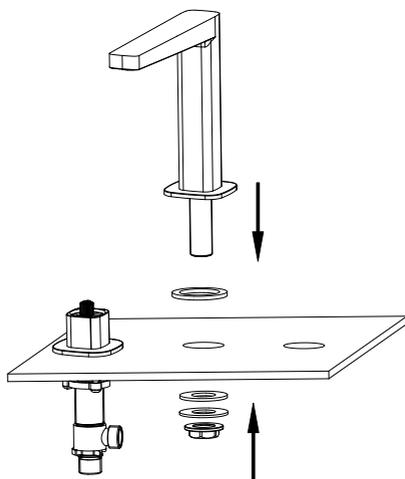
Install the spout. Make sure it is in the proper direction.
