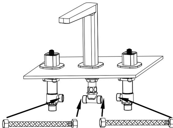
Connect the 3-way valve, hot valve, and cold valve by the flexible hoses.
