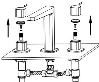
In case the handle cannot be adjusted to a proper direction. Please remove the handle, and loosen the screw in the cartridge. Take the plastic screw off from the cartridge and turn 90 degree. Please re-install every part afterward and install the handle to see if the direction is correct.
