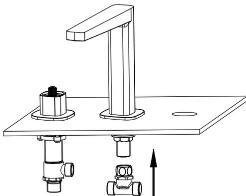
Install the 3-way valve, Make sure it is in the proper direction.
