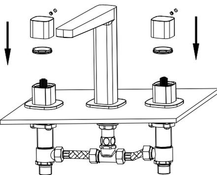
Install the hot water and cold water handle. Make sure the handle is in the proper direction.
