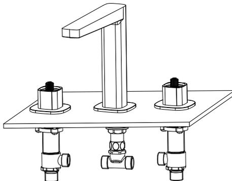
Install the valve for cold water, and tighten up the cover of the cartridge. Make sure the cover is in the proper position.
