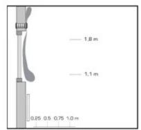
Outdoor temperature: +/- 0°C Indoor temperature: +20°C Airflaw; 8 l/s Capacity of radiator: 400 W
