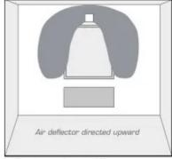
Outdoor temperature: +/- 0°C Indoor temperature: +20°C Airflow: 8 l/s Capacity of radiator: 200 W
