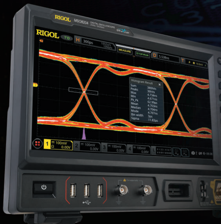
Perform eye measurement on the 622 Mb/s signal.
