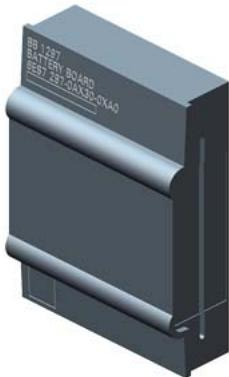
SIMATIC S7-1200, Battery Board BB 1297 for long-term buffering of the real time clock, plug-in in the signal board receptacle of the S7-12XX (FW3.0 or higher); Battery (CR1025) not included in scope of delivery
