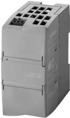
Compact Switch Module CSM 1277 for connecting SIMATIC S7-1200 and up to 3 further nodes to Industrial Ethernet with 10/100 Mbit/s; unmanaged switch, 4 RJ45 ports, ext. 24 V DC power supply LED diagnostics, S7-1200 module incl. electronic Equipment Manual on CD-ROM.
