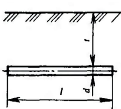
$$\left| \begin{array}{l} R = \frac{\rho}{2\pi l} \ln \frac{l^2}{dt} \text{ --- цилиндр} \\ R = \frac{\rho}{2\pi l} \ln \frac{2l^2}{bt} \text{ --- полоса} \\ \text{шириной } b \end{array} \right.$$
