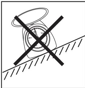
Put the scale on a firm and stable horizontal surface.
