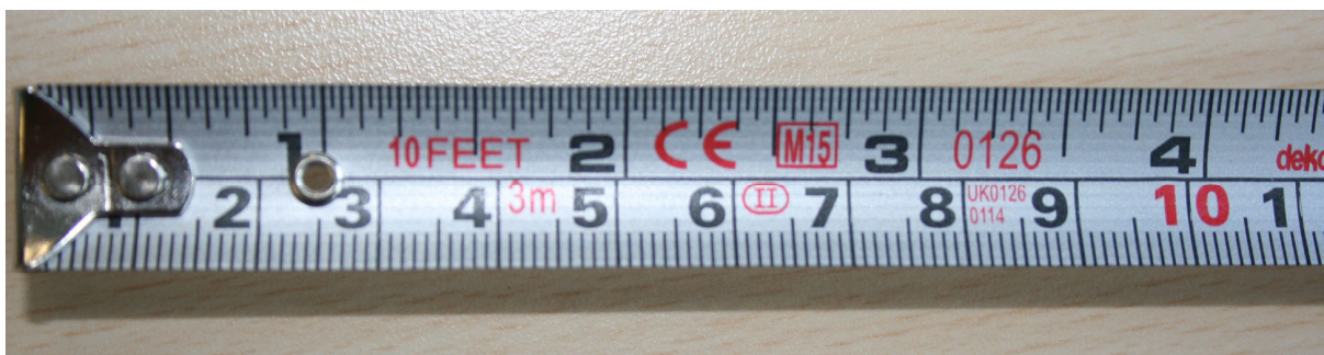
Figure 3 Example of the dual marked tape blade
