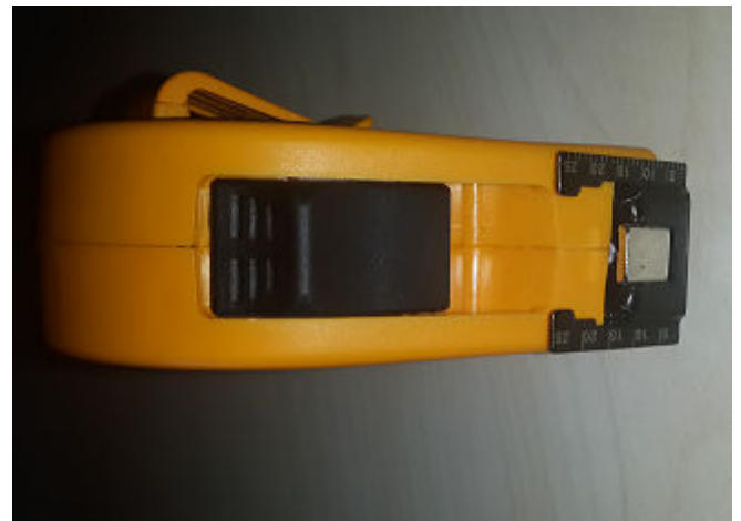
Figure 7 Example of magnetic, graduated hook (7.5)
