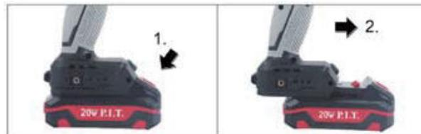
To remove the battery, press the unlocking To remove the battery , press the unlocking button and pull out the battery toward the front.
