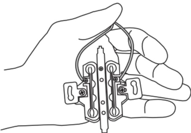
Connect the wires by pushing the skimmers into the grooves of terminals clamps. If there is a grounding wire, connect it to the appropriate contact. Tighten the screws.
