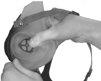
Figure 2 – Removing the protective screen of the half mask
