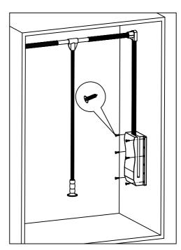
1. Use 8 pcs st4\*20 sink head screw to fix the buffer system according to schematic diagram of installation
