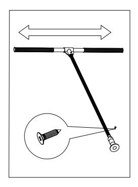
3. Use st3\*10 pan head screw to fix bar and handle, adjusting hanger rod to suitable width
