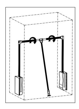
5 Adjust the bar to the suitable postion and revolve it till tighten point according to direction of photo showed. Then fasten the hexagan head screw
