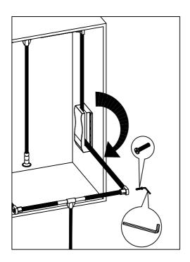
4. Pull down the wardrobe lift and install conntector and hanger rod as photo showed, and fix them by M8\*35 hexagon head screw
