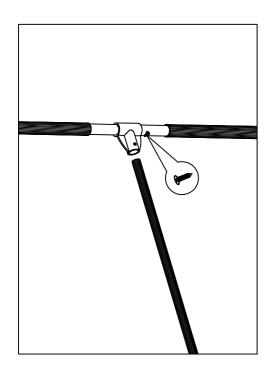
2. Use st3\*10 pan head screw to fix the bar and hanger rod
