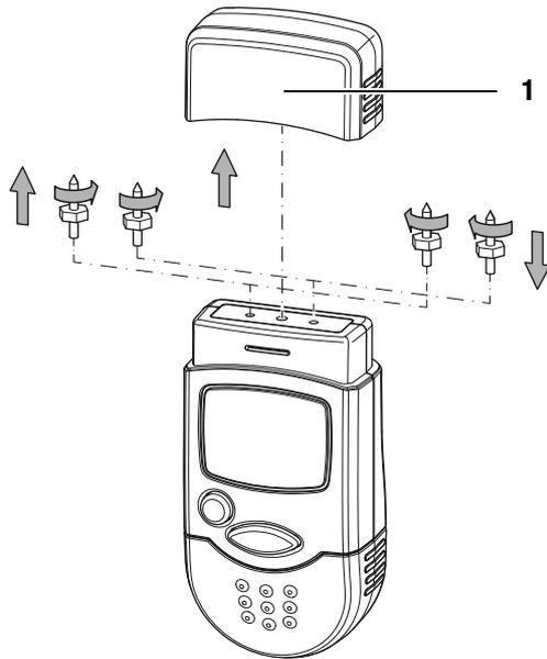
1. Remove the protective cap (1) from the device.
