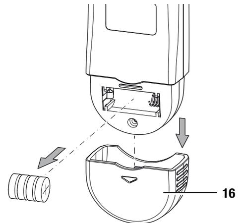
1. Remove the cover (16) from the device by sliding it in the direction of the arrow.
