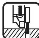
**CUTTING:** Under no circumstances should a cutting disc be used for roughing work. When cutting, do not press, tilt or oscillate.
