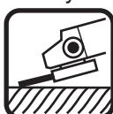
**GRIDING:** The best results are achieved with an angle of 30° to 40° for grinding, 15° for finishing. Move the machine back and forth with light pressure. In this manner, the workpiece does not become too hot, no discoloration occurs and no ridges are produced.
