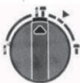
drilling with impact
