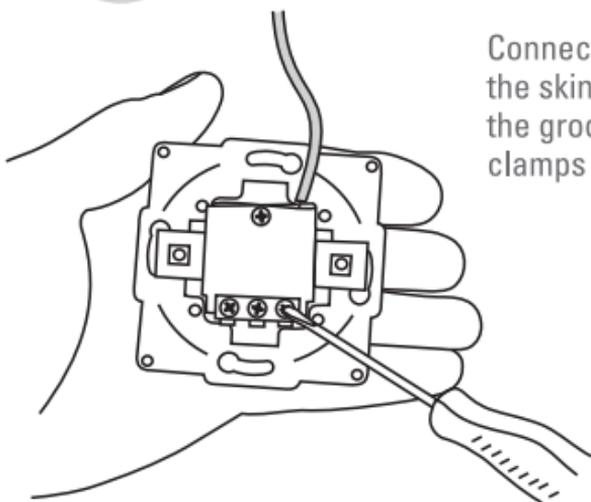
Connect the wires by pushing the skimmers (Fig. 3.1.) into the grooves of terminals clamps and tighten the screws.
