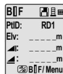
Go to menu set "Intermediate Sight" to ON OR press Height & Distance key, measure to intermediate sight
