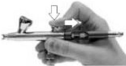
Press trigger to deliver air.
