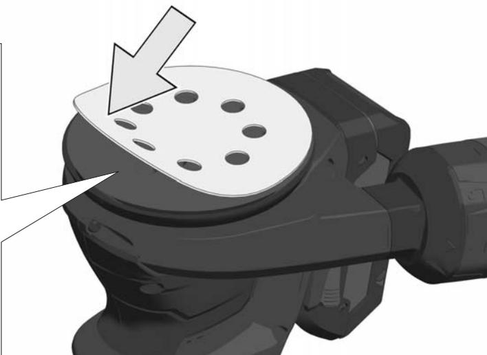
Press carefully the fuzzy side of sanding disc against the packaging pad, as firmly as possible.
