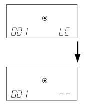
When the display appears as shown above, hold down [ON/OFF] for 2 seconds each time.
