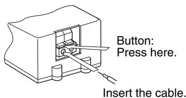
3. Connect the cable to the terminal board at the bottom rear of the Lossnay M-NET remote controller unit.
