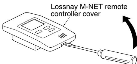
4. Remove the Lossnay M-NET remote controller cover using a standard screwdriver. Attach the Lossnay M-NET remote controller unit to the switch box using the two enclosed cross-recessed pan head screws. Use a standard screwdriver with a blade that is 4 mm or wider to remove the cover.
