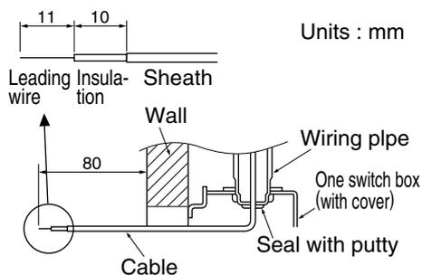
1. Pull out approximately 80 mm of cable from the wall and remove the insulation at the end.
