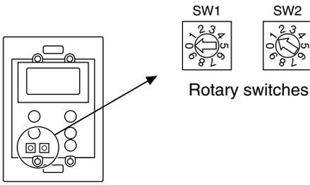
5. Set the Lossnay M-NET remote controller address.
